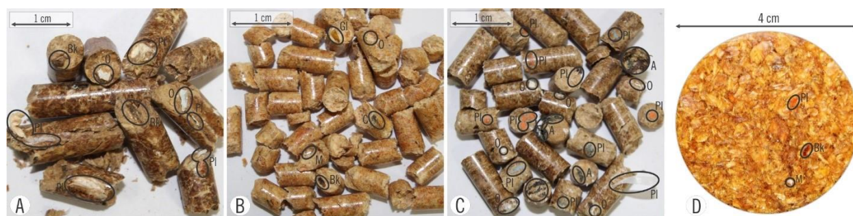
Figure 1. Wood pellets having very high contents of impurities that are visible megascopically in raw samples (A–C) and a microscope plug (D). A = ash, Bk = bark, C = coal, Gl = glass, M = metal, O = binder, Pl = plastic.
