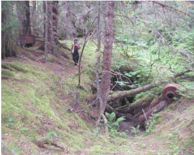
Figure 4. A view looking into the partially collapsed and flooded shaft at the coal mine locale, Kootznahoo Inlet, Alaska. Note the coal cart in upper left. Sue Karl for scale. T. White photo.
