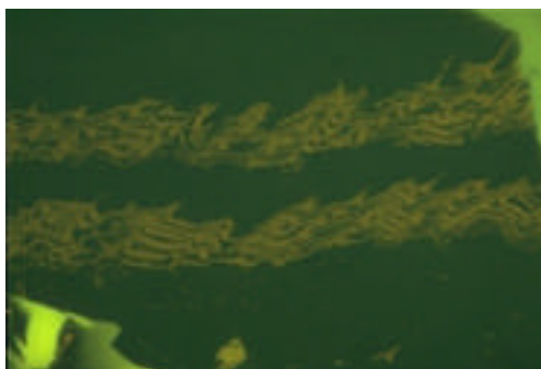
Suberinite and exsudatinite (bottom left), fluorescence mode, field width = 0.30 mm
